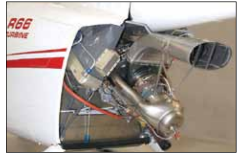
The Rolls Royce RR300 turboshaft engine was specifically designed for the R66.
